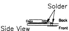
Scrape off Solder Mask Here or Here to solder the Coax Shield
